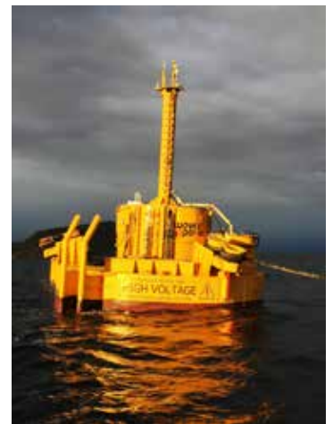
Buoy used to generate electricity from waves
